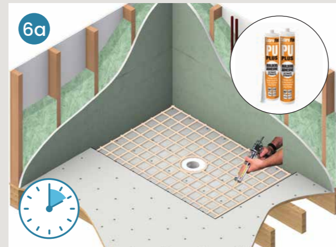
6a Tile & Slate Floor - Apply polyurethane adhesive. 2hr cure time (adhesive kit included)
