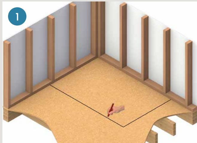
1 Mark outline of base on timber floor
